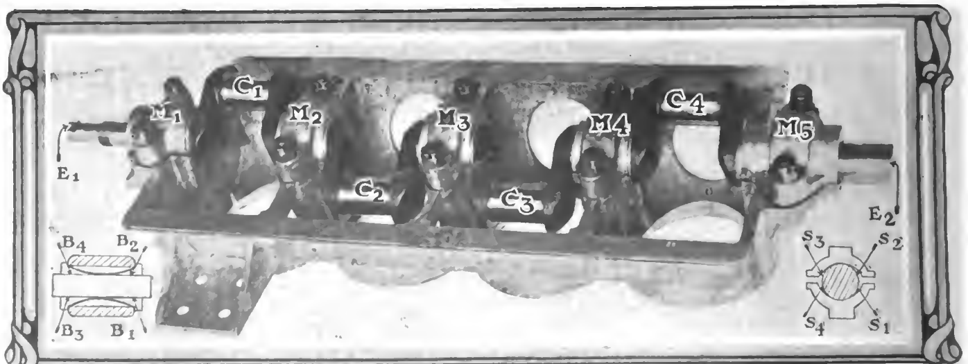
Fig. 3—Crankshaft in place after bearings were scraped in and liners reduced to requisite thickness to let cap down to contact
